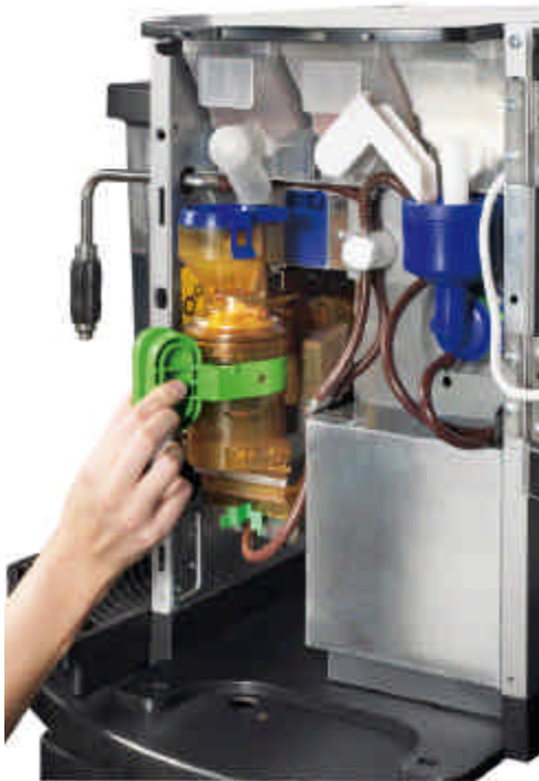
DETAIL OF BREWING CHAMBER BEING REMOVED
