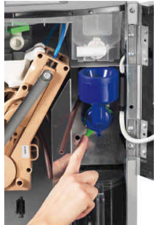
MIXER IN EXTRACTION POSITION: DETAIL OF RELEASE LEVER
