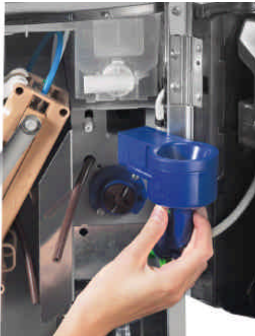
MIXER HAVING THE EXTERNAL PARTS THAT NEED DAILY HYGIENE BEING REMOVED
