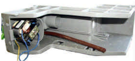
MIXER RATIOMOTOR ASSEMBLY VIEWED FROM BELOW
