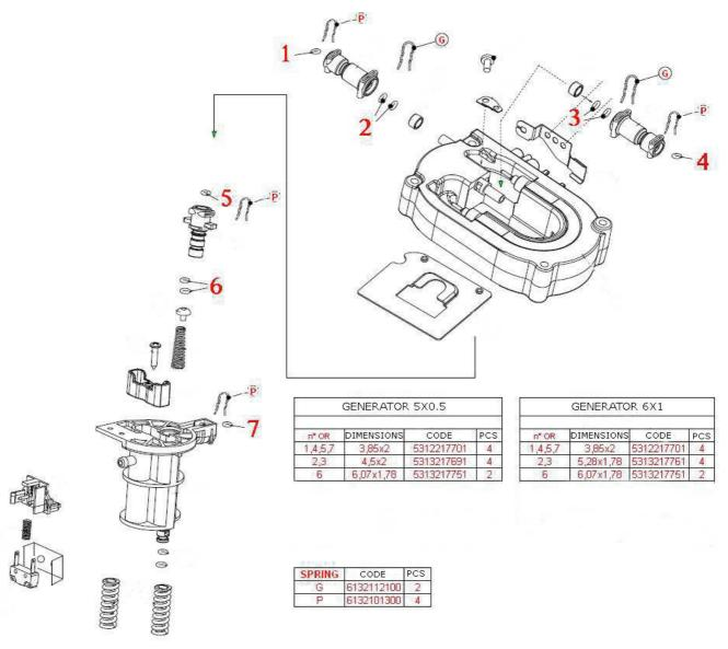
Please note that to replace the o-ring from **1-5 and 7** is enough to disconnect the tube and riconnect it afterwards. Pay particular attention when replacing the **2 o-rings 6** following the annexed procedure.
