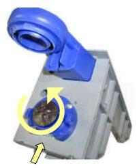
Unscrew the impeller anticlockwise, holding the knurled nut with a finger
