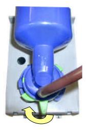
Rotate the yellow lever anticlockwise
